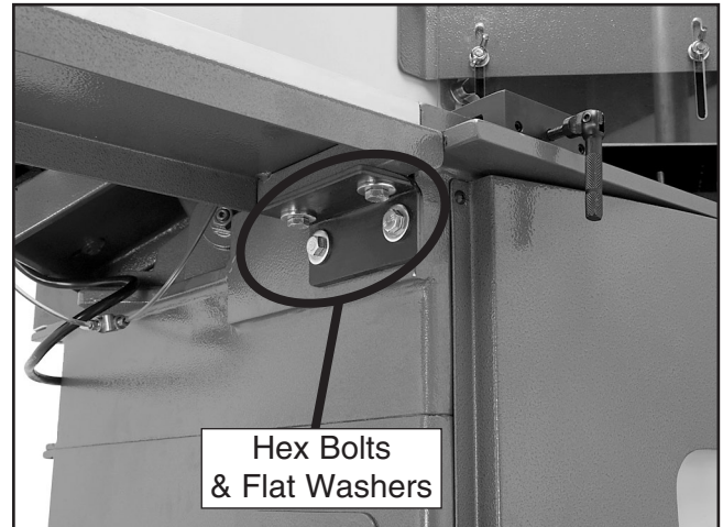
Figure 10. Extension wing mounted onto the saw table.
